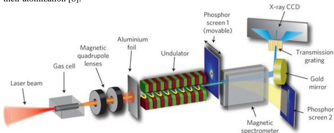
**Fig. 1 Example of the experimental setup with gas cells [9].**
