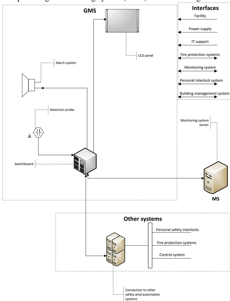
**Fig. 3 Possible setup of the monitoring system.**
