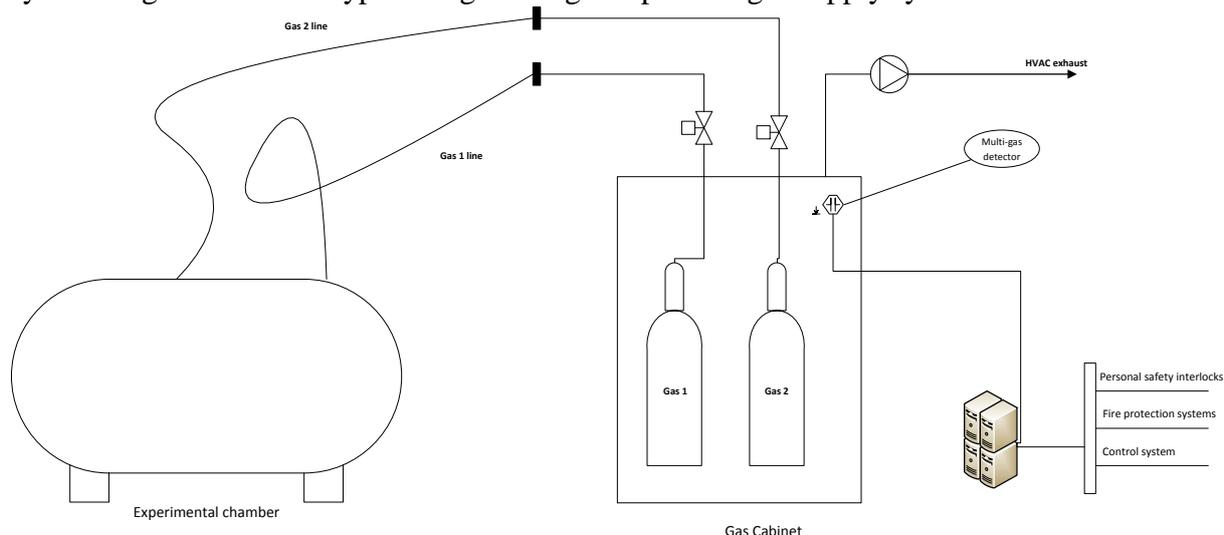
**Fig. 2 Typical design of the gas supply system.**
